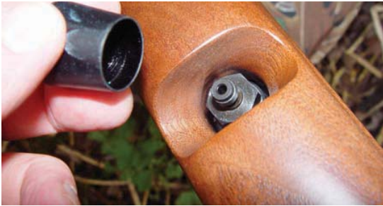
The buddy bottle is filled in situ using the quick fill connection recessed into the under side of the forend
