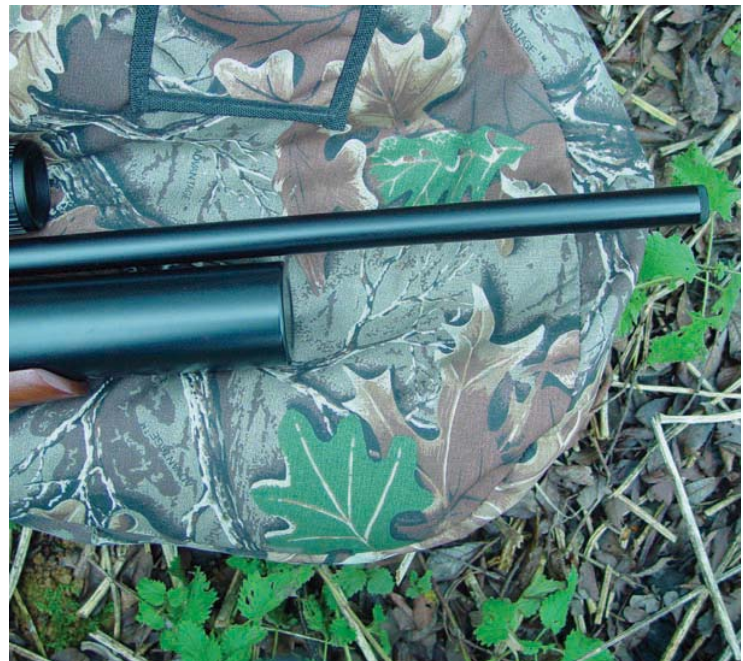
The bull barrel conceals an extremely effective sound moderation system; note also the 400cc buddy bottle – a larger bottle is optional
