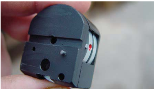
Daystate's 10-shot magazine – the slot locates the magazine and the reversible pin stops it passing right through the receiver
